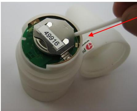
The battery is gently pressed out of the holder, for example with a cotton swab or a match.
