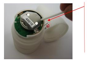
The battery is gently pressed out of the holder, for example with a cotton swab or a match. **Never use a metal object.**
