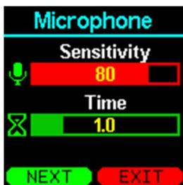
Sensitivity can be set between 0 - 100% and the activation time 0 - 5.0 seconds.
